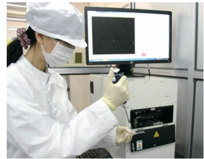
Figure 1. Device Configuration of a Microfluidic Chip-type Nanoparticle Analysis System
